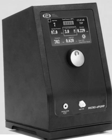
The MICRO-ePUMP is designed to inject very small quantities of fluids, such as drugs, into cells or small organelles. WPI's MICRO-ePORE™ Pin-point Cell Penetrator technology is embedded inside the MICRO-ePUMP. When the researcher enables the MICRO-ePORE™, it delivers a highly localized voltage signal to a targeted injection site to facilitate penetration with minimal trauma.
