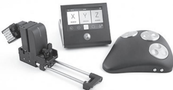
Extreme stability and accurate positioning due to piezo-driven movement over 20 mm range with 5 nm resolution. 3-axis and 4-axis versions, touch screen controller and rotary wheel remote interface.
