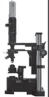
Easy removal of transmitted light pass System and raise of Objective / Epifluorescence high allows to adapt any kind of InVivo system like Jetball or Treadmill.
